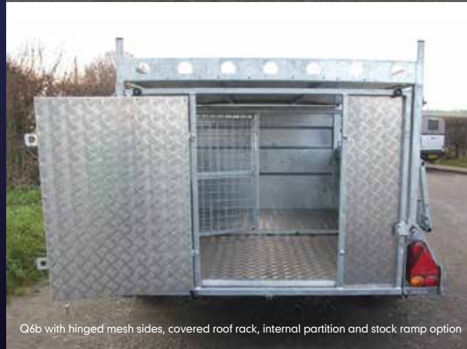
Q6b with hinged mesh sides, covered roof rack, internal partition and stock ramp option
