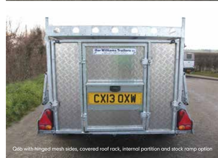
Q6b with hinged mesh sides, covered roof rack, internal partition and stock ramp option
