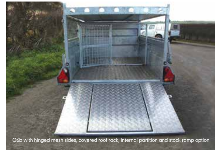
Q6b with hinged mesh sides, covered roof rack, internal partition and stock ramp option
