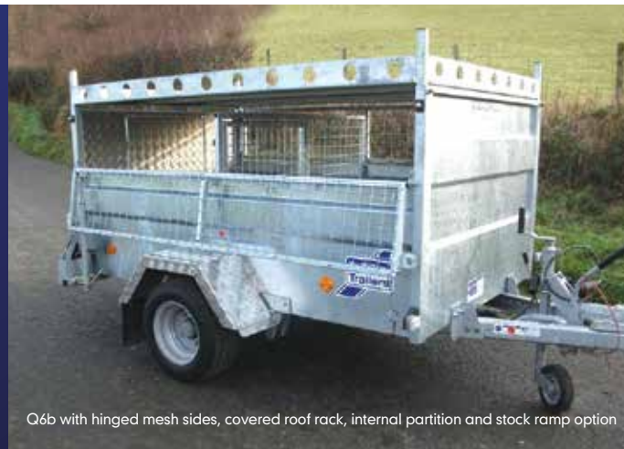
Q6b with hinged mesh sides, covered roof rack, internal partition and stock ramp option
